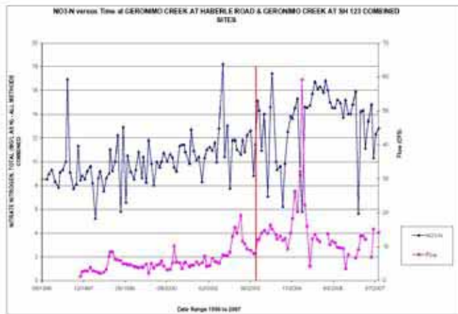
Figure 6. Nitrate nitrogen versus time at the combined Geronimo Creek at SH 123 (14932) and Haberle Road (12576) stations. The vertical red line represents the transition from the SH 123 (14932) and Haberle Road (12576) station.
