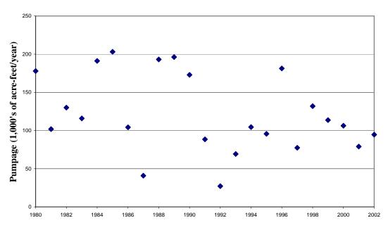
Figure 3.3-3 - Total Irrigation Well Pumpage
