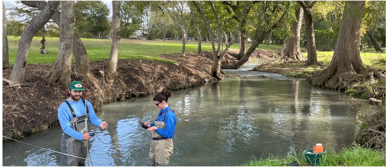
GBRA Water Quality Team Conducting Flow Measurement on Geronimo Creek
