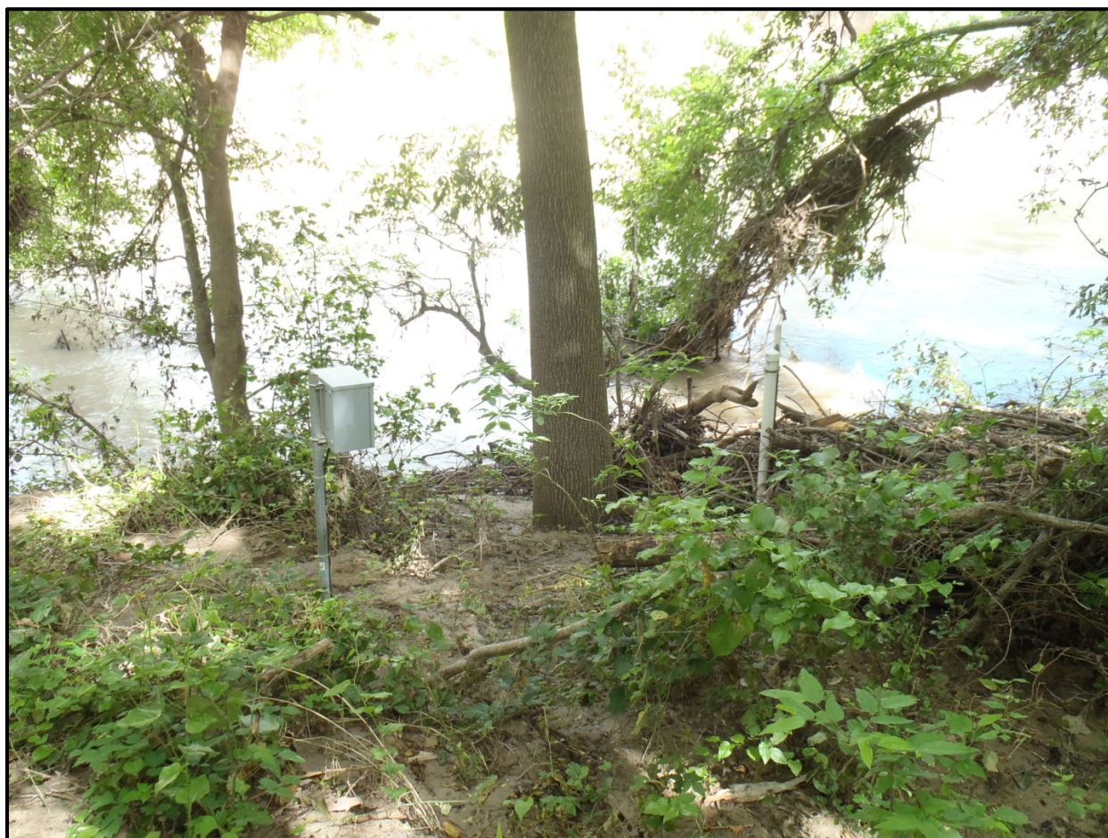
Figure 15. Soil moisture recording equipment (left) and crest stage gage (right) along a riparian transect.
