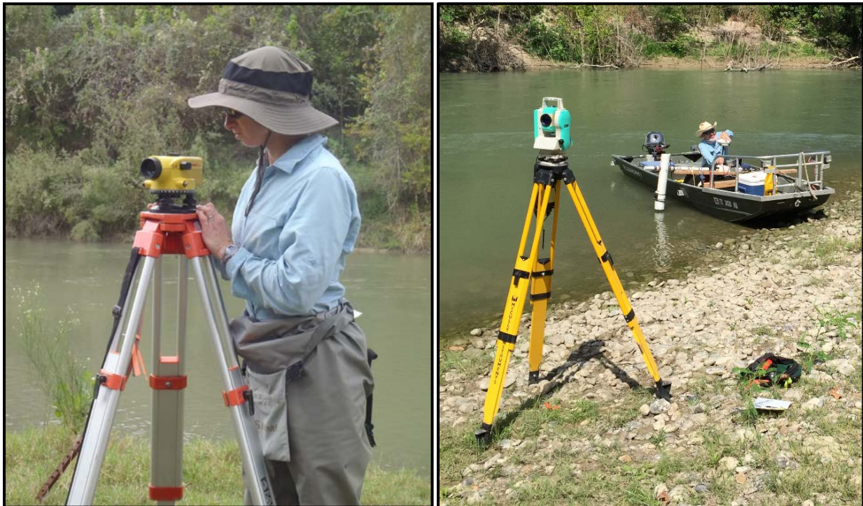
Figure 7. Surveying water surface elevations from established benchmarks using autolevel (left) and total station (right).
