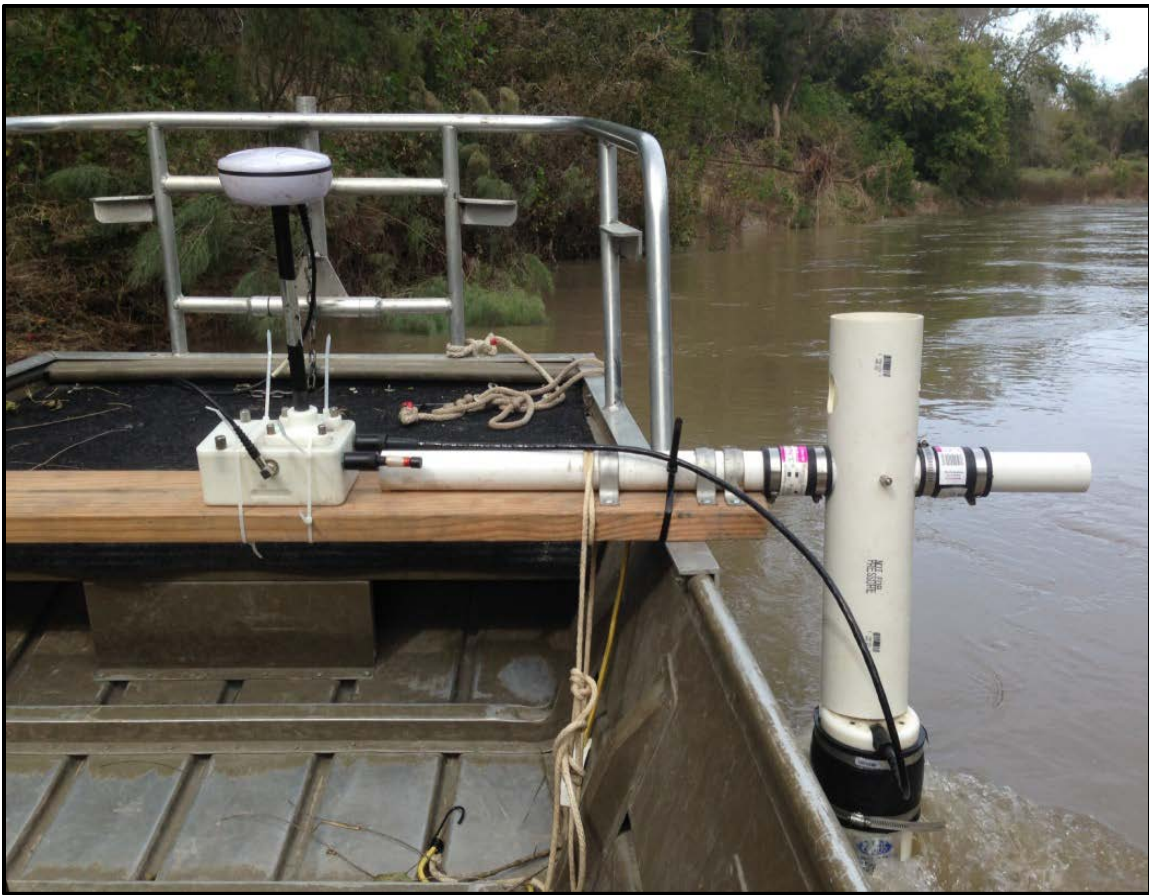
Figure 3. SonTek M9 River Surveyor mounted on a small john boat.
