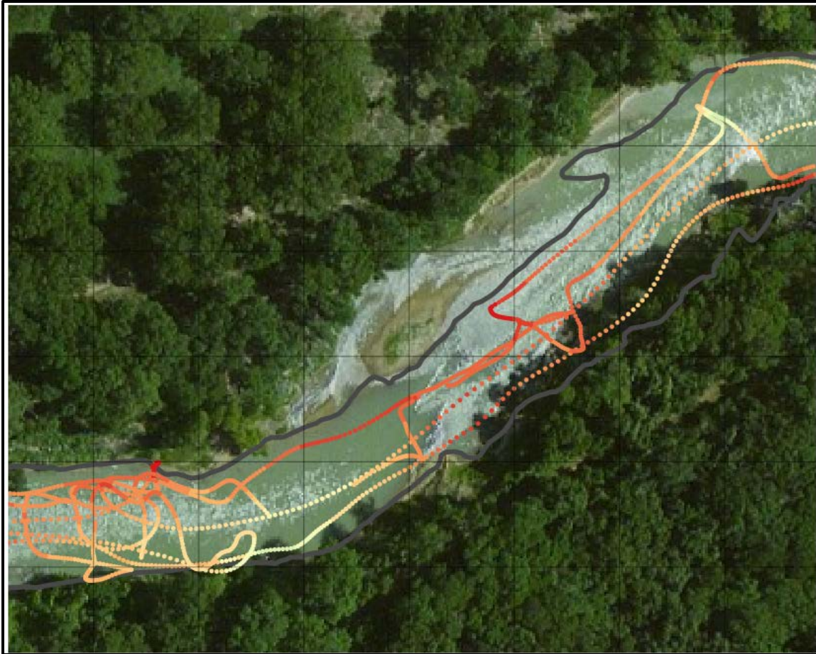
Figure 6. Site excerpt with M9 echosounder points collected in September 2015.
