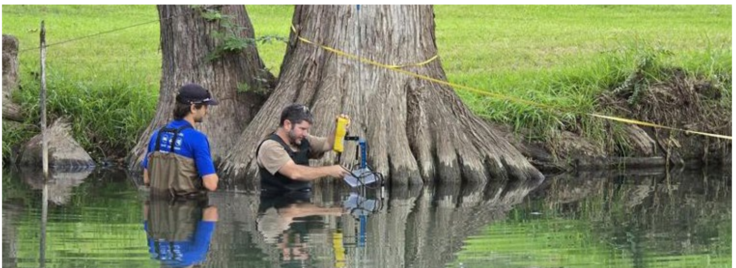
Measuring flow on the San Marcos River.
